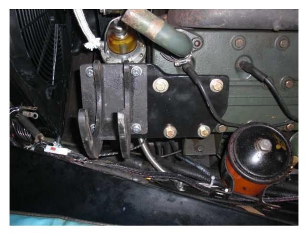
Notice the plate required a cut-out to clear the #1 sparkplug opening, and another to clear the 3rd lower head bolt.
