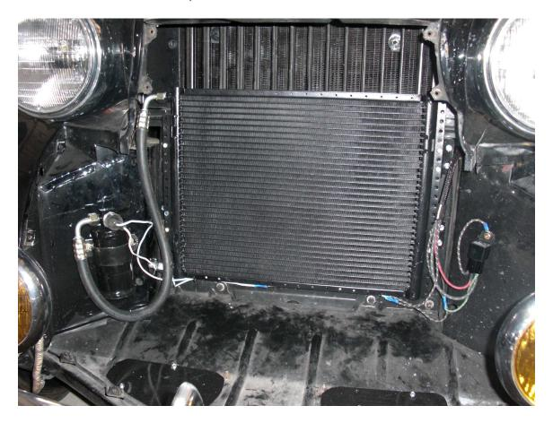
While behind the grill, I fabricated a pair of "block-off plates" to cover the air openings in the bottom of the pan. My guess is these are here to allow a place for air to escape when the cooling louvers are closed. In Texas summers though, I want every cc of air to be forced right through that radiator:
